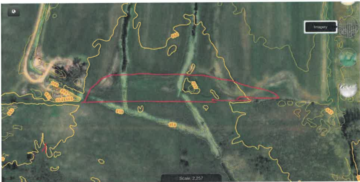
Figure 1. Red outline shows the approximate area of proposed excavation. Surface contours are in two foot intervals.
